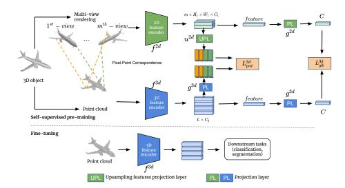
Fig. 1: Overview of our proposed method. The main proposal is pre-training steps that exploit multi-modal data, including multi-view images and point clouds, to learn a 3D feature encoder for effective point cloud representation. This model is then fine-tuned for different downstream tasks.
